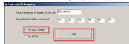
2. Enter a temporary IP address for the IPI-4 that does not conflict with any other components on the network. Next; enter the MAC address of the adapter in the provided fields.
